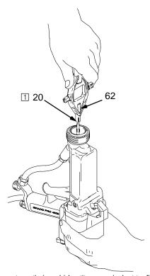
Apply low-strength (purple) Loctite or equivalent to fluid rod threads
